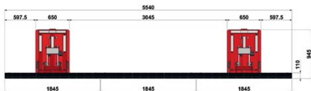
Barrier with three elements: two closed, one lowered. Access width: 3 metres.
