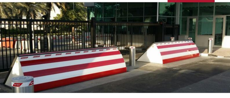
ARMIS Roadblocker RB500 are built «shallow mounted». That means they only require a 300 mm foundation depth. This allows easy and cost-effective installation, independent of existing facilities such as cable ducts, drainage systems, etc. Furthermore, ground level mounting on slopes is possible.
