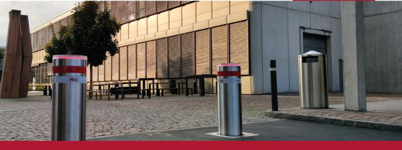
New automatic bollards with efficient and operationally reliable hydraulic drive are used both for passages with an increased traffic frequency and as simple barriers. These include traffic-calmed zones, pedestrian areas or bus lanes. Different types of control on control pillars, or installed on walls or booths allow simple, intelligent control.
