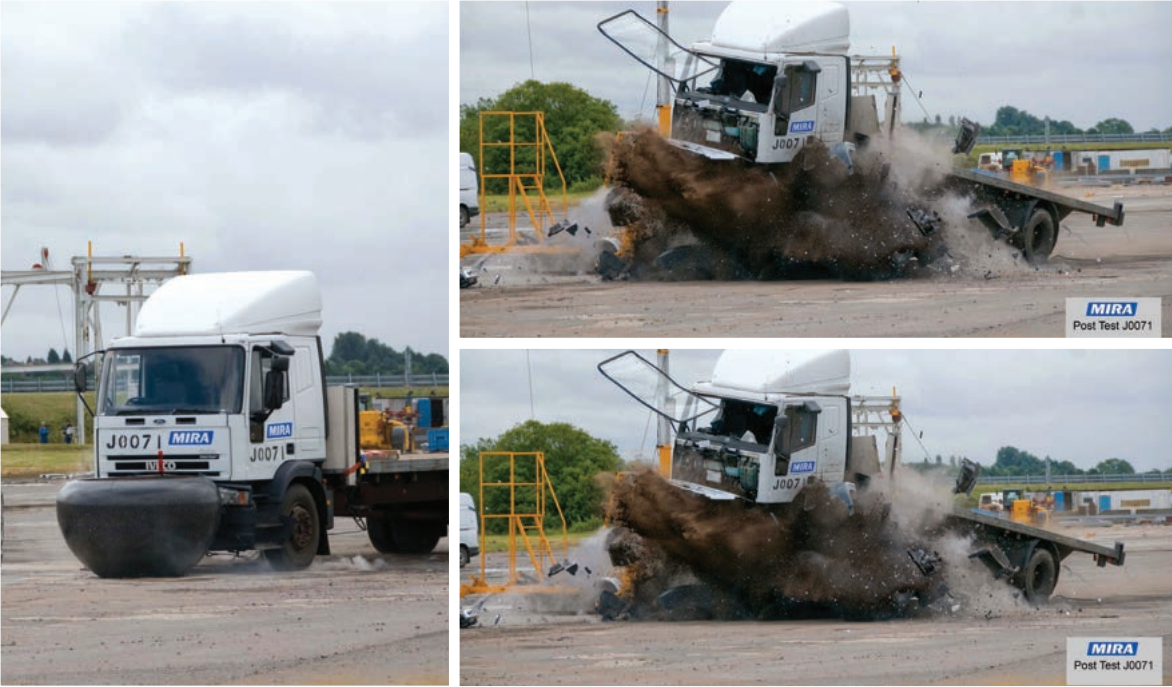
RhinoGuard® Glove Planter crash test
