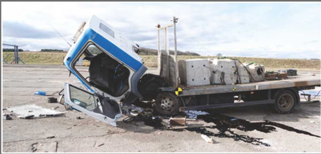
IWA14.1-1:2013 Bollard, Performance Rating: V/7200(N2A)/64/90:7.6
